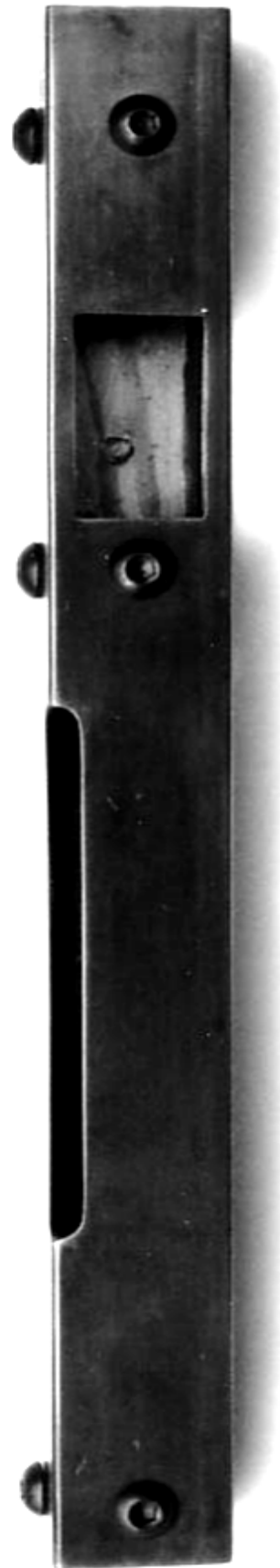
Photo 28: Three collars fitted to the receiver.
