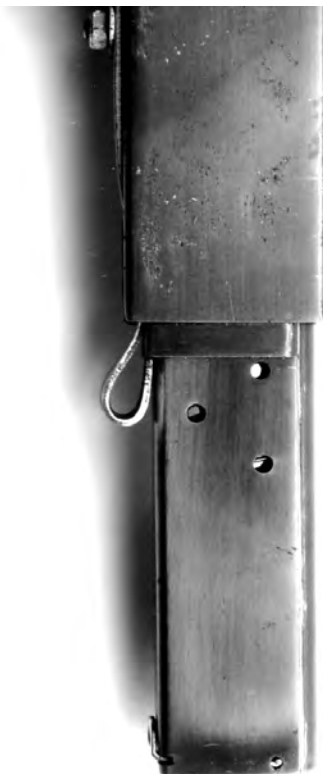
Photo 15: The spring catch holding magazine in place.
