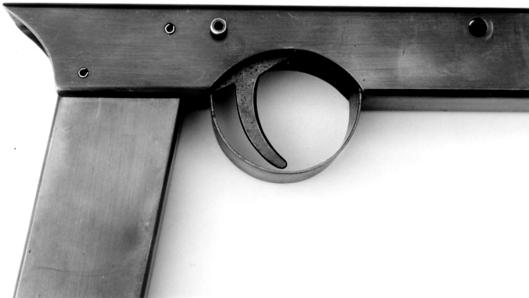
Photo 17: Trigger and guard fitted to receiver
