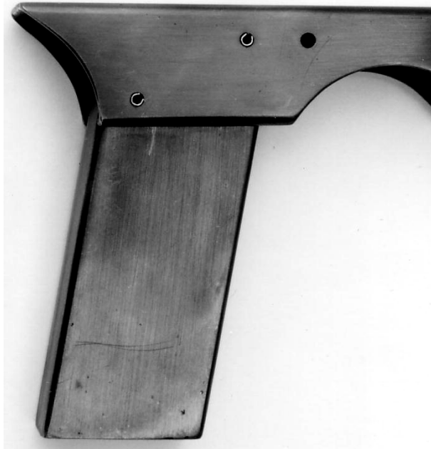
Photo 6: The grip pinned in position
