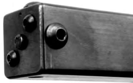
Photo 39: The recoil shield fitted to receiver.
